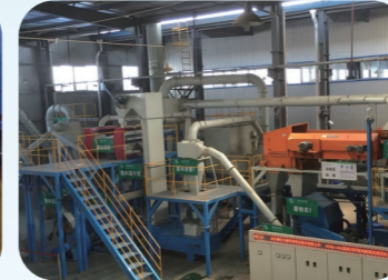
废线路板一体化物理破碎设备 生产线 Integrated physical crushing equipment for waste circuit boards
